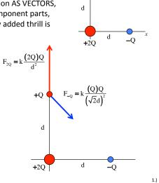
Breaking the off-axis force into components requires an angle. Ignoring the fact that the angle is really 45°, we can define it generally as  $\theta$  (see sketch) and, looking at the physical triangle that exists in the sketch, note that:
